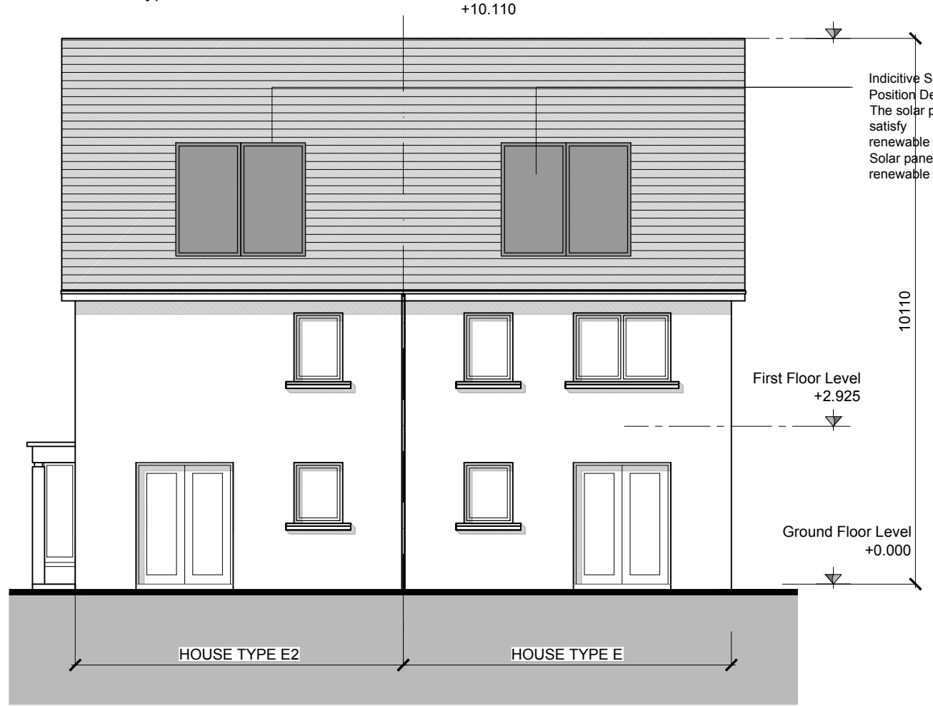
REAR ELEVATION House Type E-E1 - Semi Detached
