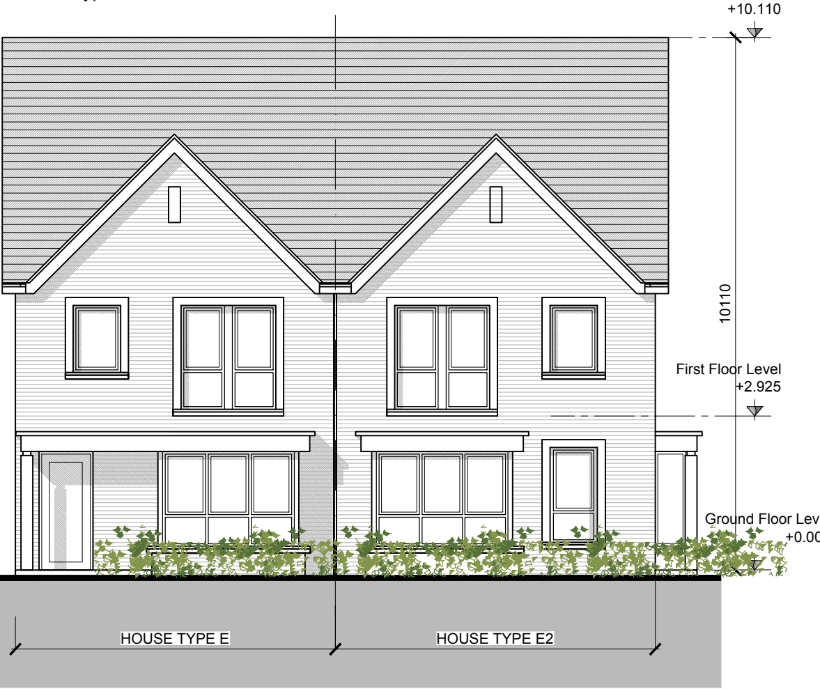
FRONT ELEVATION House Type E-E1 - Semi Detached
